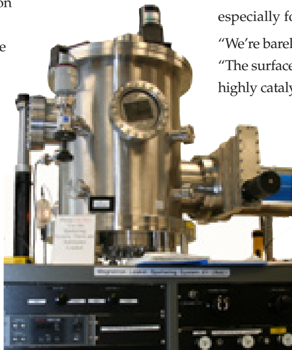
A sputter machine used to produce nanoparticles. Photo credit: NanoFab at University of Alberta
